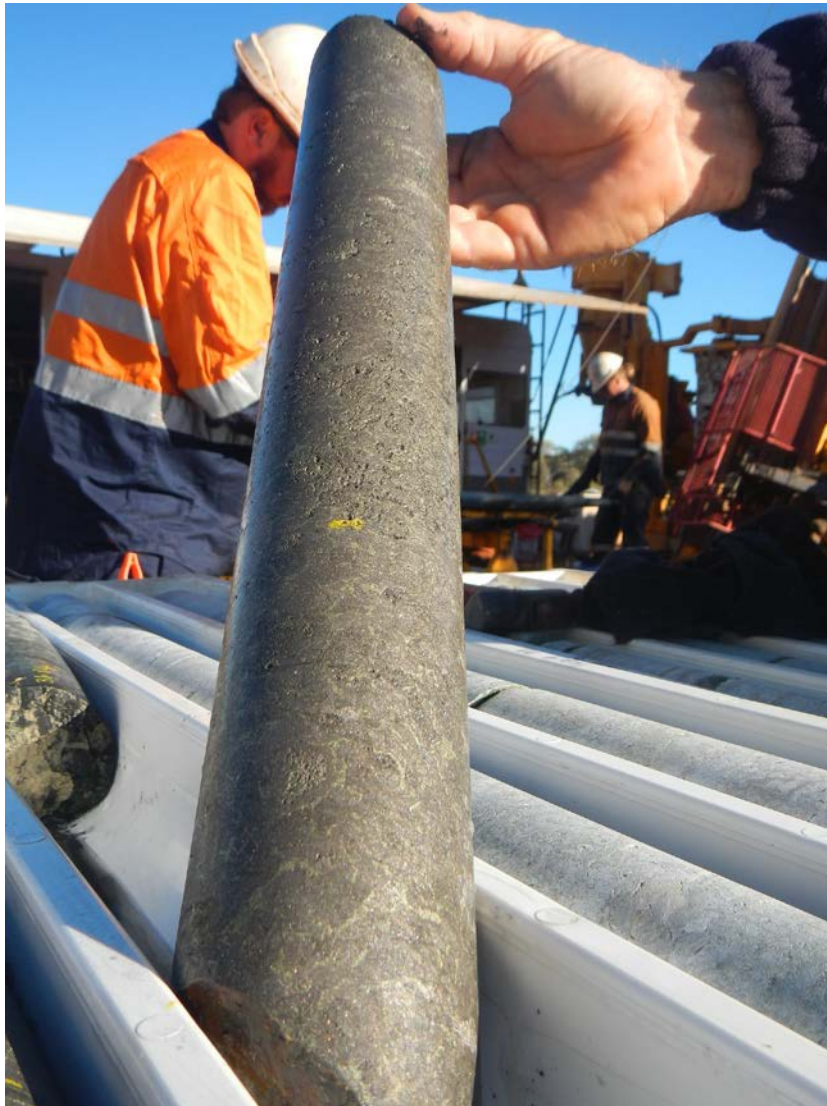
Figure 1 – photograph of drill core from MAD15 interval between 30.17m to 31.34m. Core comprises massive nickel-copper sulphides (pentlandite, chalcopyrite) with average 8.9%Ni and 3.2%Cu (based on XRF analysis)
