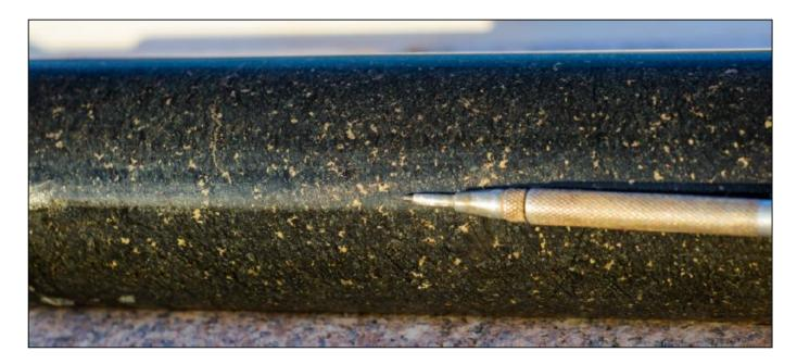
**Figure 1:** Drill-core with heavily disseminated sulphides from the interval at 46.3m to 48.7m downhole in MAD152 at the Radar Prospect
