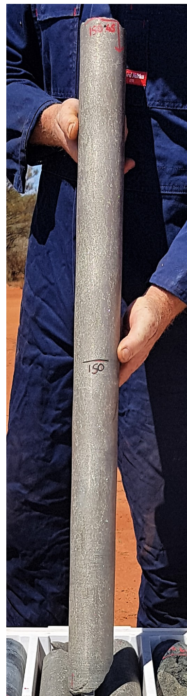
Above: photo of drill core from the massive sulphide interval of MAD136 between 149.55m to 151.93m with average XRF readings of 8.1%Ni and 3.21%Cu*
