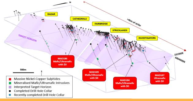
Left: Schematic orthographic view of the Cathedrals Belt showing the large interpreted target horizon which dips to the north-west at approx. 40 degrees. Shallow drilling and known shallow massive nickel-copper sulphides are also shown.
