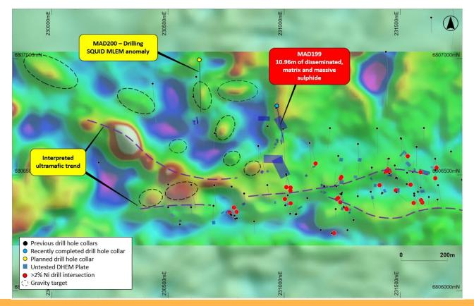
Plan view map of West End and Investigators showing recent gravity survey data (25m spacing) and prior drilling. Gravity highs are targets for potential areas of nickel-copper sulphides.
