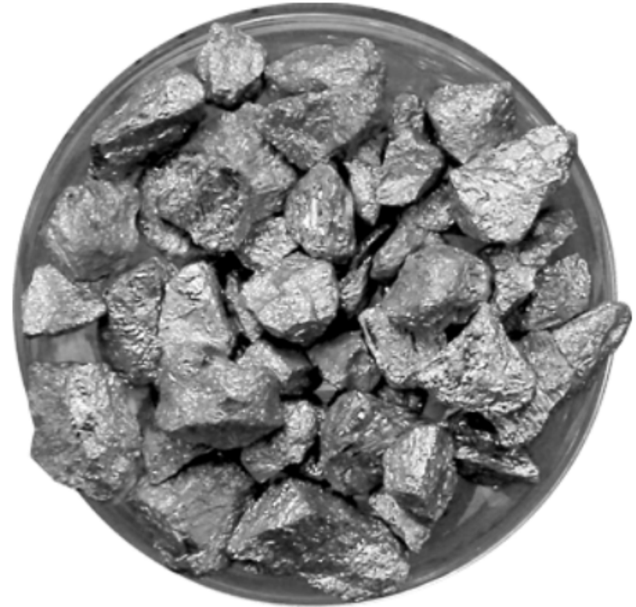
Ferroniobium produced at the CBMM niobium facilities 3
