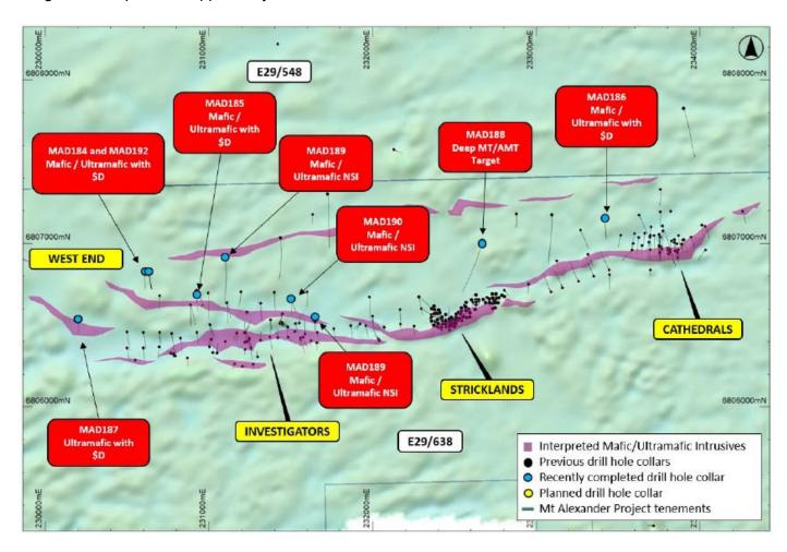
**Figure 2:** Plan view of the Cathedrals Belt showing areas of recently completed and planned drilling, overlaying interpreted geology and magnetics (TMI RTP 1VD).
