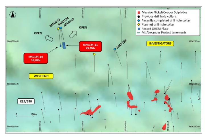
**Figure 1:** Plan view of the western part of the Cathedrals Belt (against TMI RTP 1VD) showing the new EM conductors at the West End Prospect as well as massive nickel-copper sulphides already discovered.
