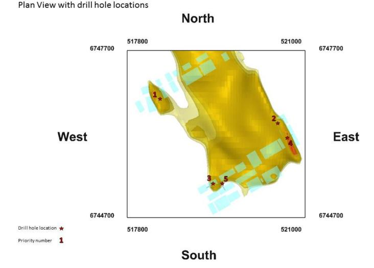
Figure 1 – a plan view of the ultramafic body with 2012 priority drill-hole locations. Hole 1 (CAMRC-001) was completed and Hole 2 (CAMRC-002) was partially completed to a depth of 150m.
