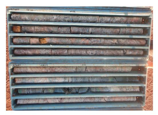
Figure 4 – MAD213 from 666.50m to 674m showing a portion of the 120m+ intersect of coarsegrained pegmatite from the Manta seismic reflector
