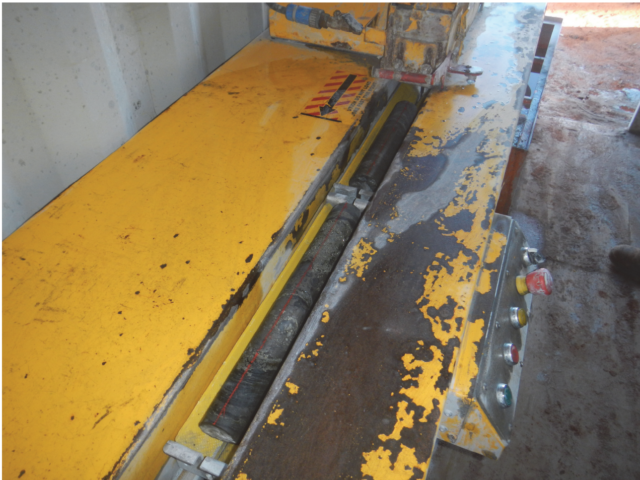
Figure 1 – cutting of the drill core at site. The first batch of laboratory assays for the sampled drill core is expected soon.
