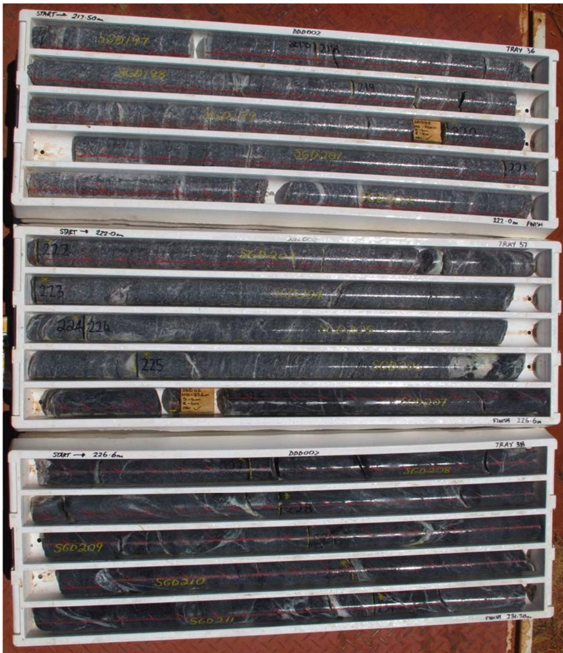
Figure 2 - Trays 36, 37 and 38 for DDD002 contain core from 217.5m to 231.3m. This is a thick ultramafic unit with an alteration assemblage of talc, chlorite, carbonate and magnetite. Laboratory assays will provide an accurate assessment of the nickel content of this interval.
