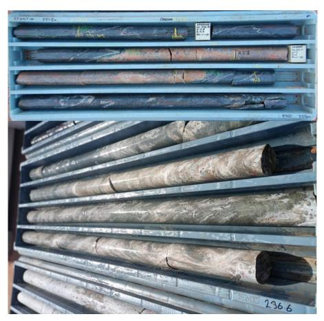
Figure 1: Core from PDD006 (top) and PDD007 (bottom). PDD006 shows large potassic altered granite dyke cross-cutting sediment package and PDD007 showing chlorite altered carbonate sediments with disseminated sulphides (see Table 2). Assays are pending.
