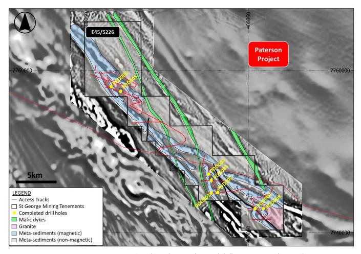
Figure 3: Paterson Project interpreted geology showing diamond drilling status overlying airborne magnetics imagery.
