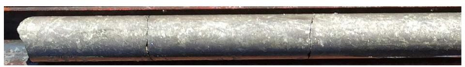
Above: part of the massive nickel-copper sulphide intersection in MAD40 that graded 7.88%Ni and 3.11%Cu
