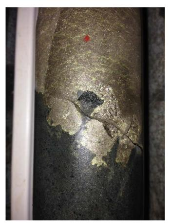
**Above**: drill core from MAD23 at 57m showing contact of massive nickel-copper sulphides against footwall mafics
