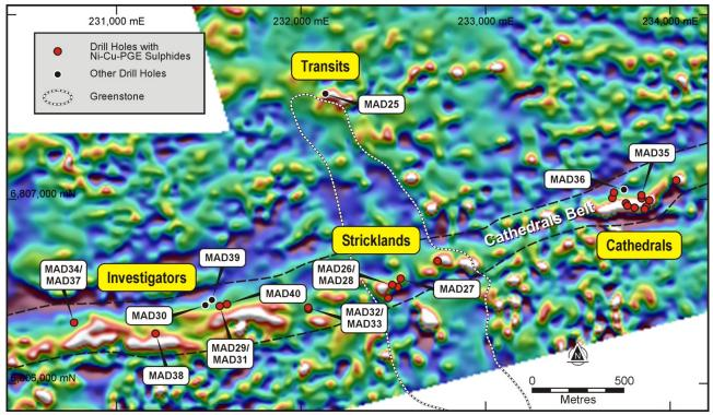
Figure 6 – a plan view of the Cathedrals Belt (over TMI magnetics) showing the drill hole collar locations in the second drill programme completed by St George at Mt Alexander. Further discoveries of nickel-copper sulphides were made at the Cathedrals and Stricklands Prospects, and new discoveries were made at the Investigators Prospect. Nickel-copper sulphides are recurrent over a 3.5km strike length.
