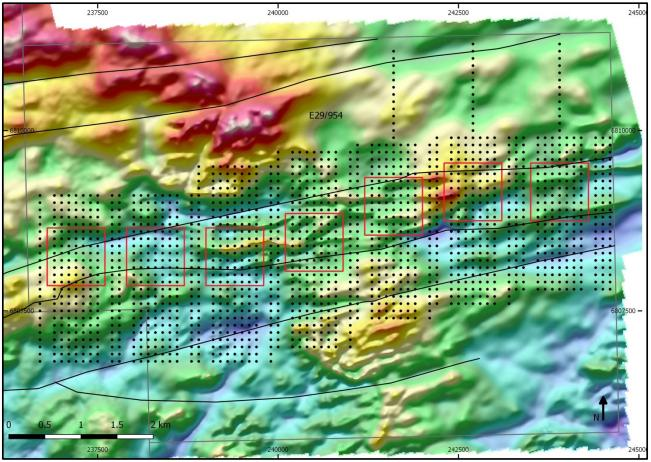
Figure 5 – a plan view of the eastern extension of the Cathedrals Belt (against TMI RTP magnetics) showing the planned EM loops (red) and north-south survey lines for the FLEM SAMSON survey over this section of the Belt.
