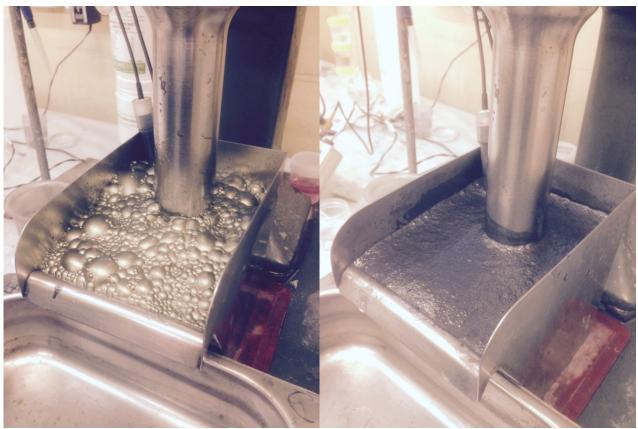
Figure 1 – photographs of a metallurgical flotation test on the Mt Alexander massive sulphide. <u>On left</u>: copper flotation test, with concentrates up to 32%Cu produced. <u>On right</u>: nickel flotation test, with concentrates up to 18%Ni produced.
