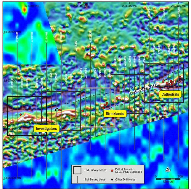
Figure 4 – a plan view of the Cathedrals Belt (against TMI 1VD magnetics) showing the planned EM loops and survey lines for the new FLEM survey over the western section of the Cathedrals Belt. Nineteen diamond drill holes completed in 2016 by St George over this part of the Belt intersected high grade nickel-copper sulphides at depths ranging from 25m to 170m. The FLEM SAMSON survey has detected new EM conductors that are deeper than the massive nickel-copper sulphides intersected to date.
