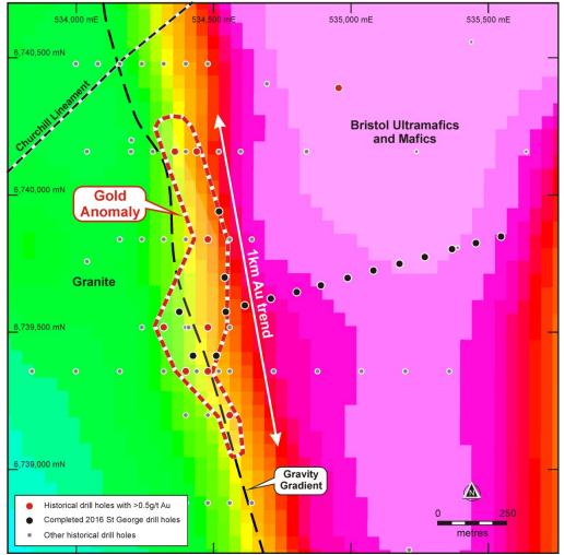
Figure 8 – the Bristol gold target (against RTP magnetics) with St George's completed drill holes shown. The gold anomalism occurs on a distinct magnetic (and gravity) gradient, a setting that is often associated with gold mineralisation.
