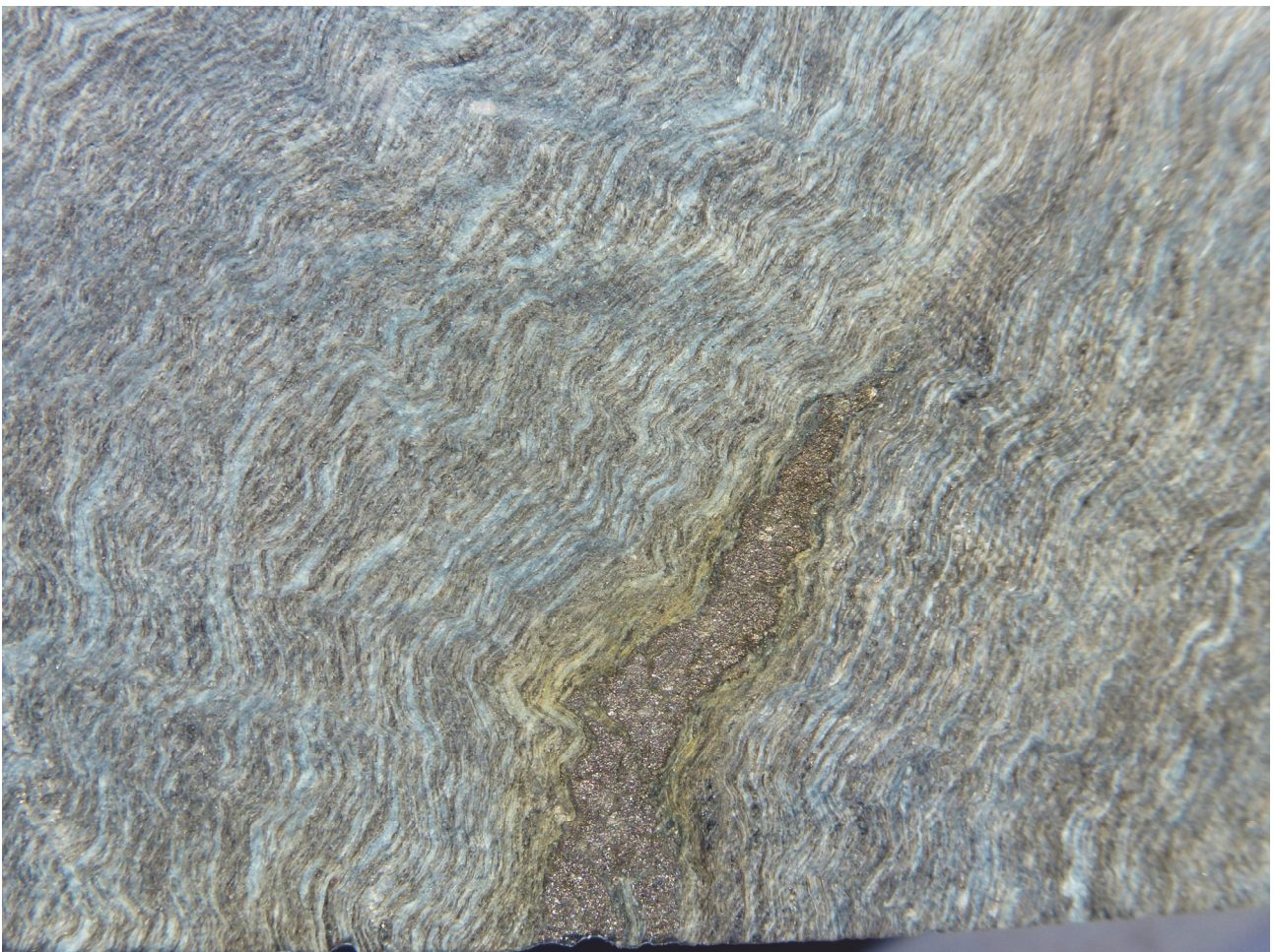
Figure 1 – a photograph of the drill core from DDRDD0005 showing a nickel sulphide stringer (3cm in length) at 237m within the sheared basal contact of the prospective ultramafic. Spot XRF analysis of the stringer sulphide recorded 1.6% Ni. The core is NQ2 size, 5cm in diameter.
