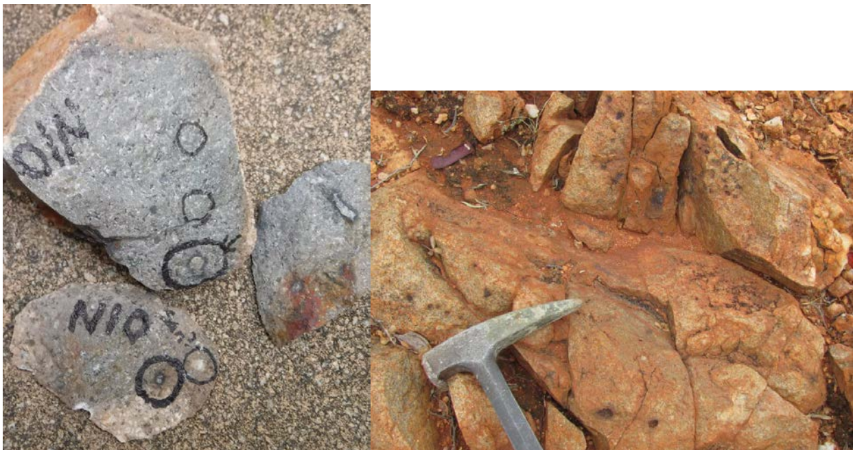
Figure 4 – specimen samples of nickel sulphide globules in outcrop at Cathedrals (GR 233420E, 6806901N).
