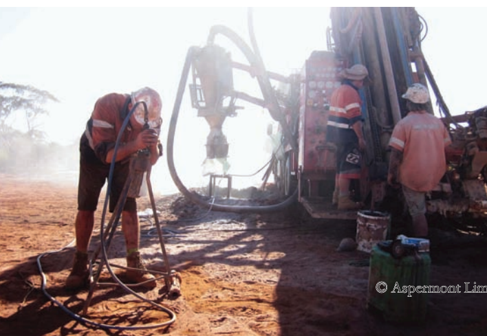
RC drilling at East Laverton.
