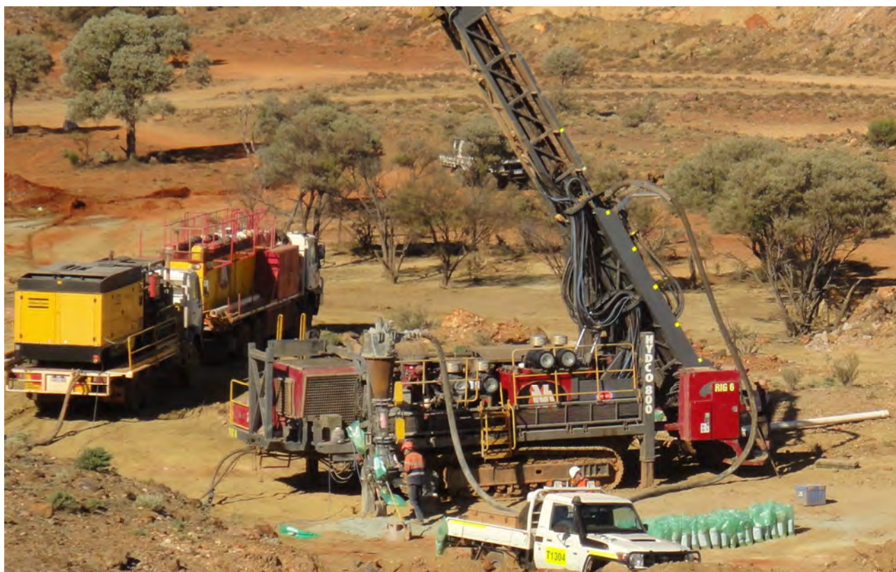
Figure 1 – a photo of a Hydco 800 drill rig that will undertake RC drilling at Cambridge
