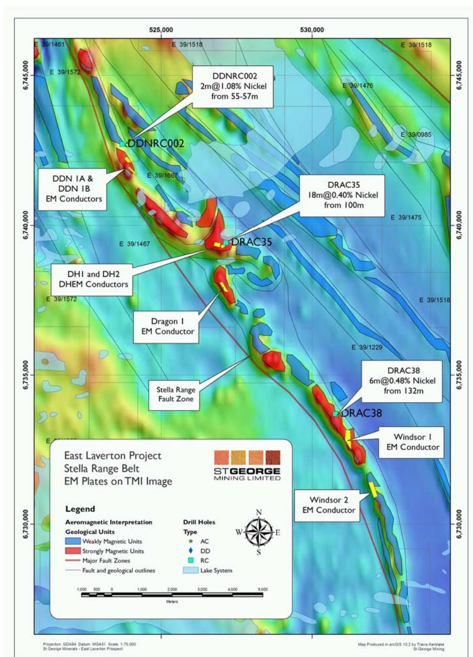
Figure 1 – Modelled EM conductors along a nickel sulphide bearing section of the Stella Range belt that hosts the Desert Dragon North, Desert Dragon and Windsor nickel prospects.
