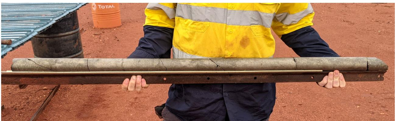
*Figure 1 – drill core from MAD199 showing massive nickel-copper sulphides 342.12m to 343.4m downhole*
