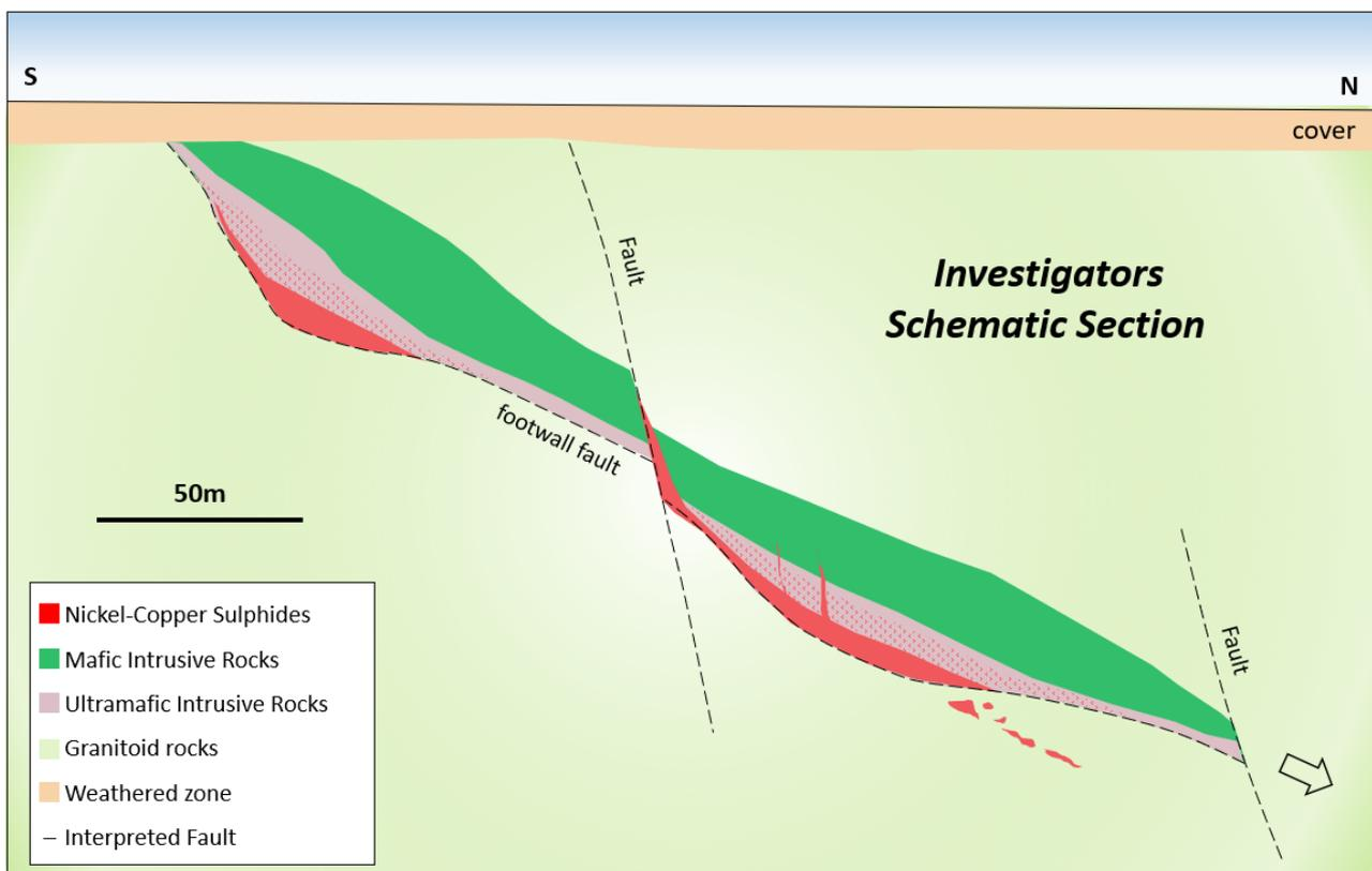
*Figure 4 – Schematic view of the Investigators Prospect (looking west) showing the generalised interpreted geology, structural features and various types of nickel-copper sulphide mineralisation intersected to date. The West End Prospect is interpreted to be a continuation of the Investigators area.*
