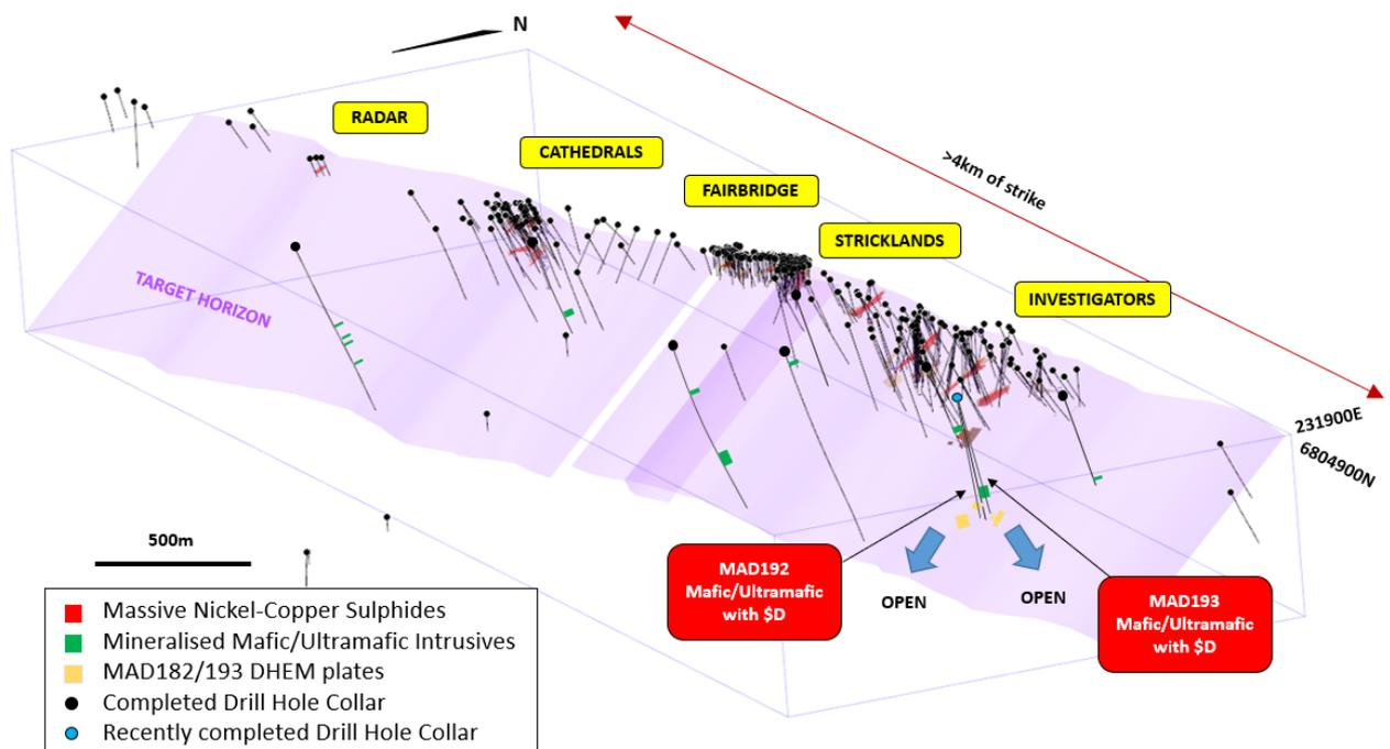
*Figure 3 – Orthographic view of the Cathedrals Belt showing the large interpreted target horizon, the new discoveries in recent drill holes including MAD192 and MAD193 as well as existing drilling and known massive nickel-copper sulphides.*
