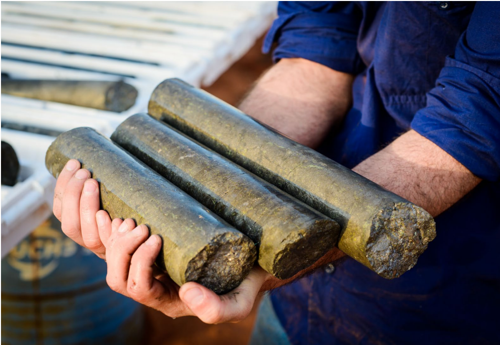
Figure 1 – drill core with massive sulphides from the interval at 49.07m downhole in MAD152 at the Radar Prospect
