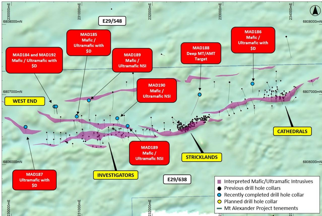
Figure 2 – plan view of the Cathedrals Belt showing areas of recently completed and planned drilling, overlaying interpreted geology and magnetics (TMI RTP 1VD).
