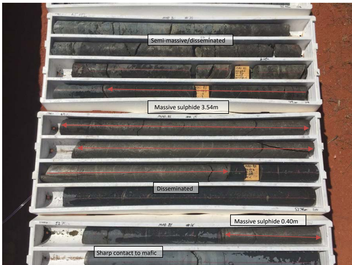
Figure 1 – drill core from MAD85 from 45.45m to 54.3m downhole showing the sulphide intervals.
