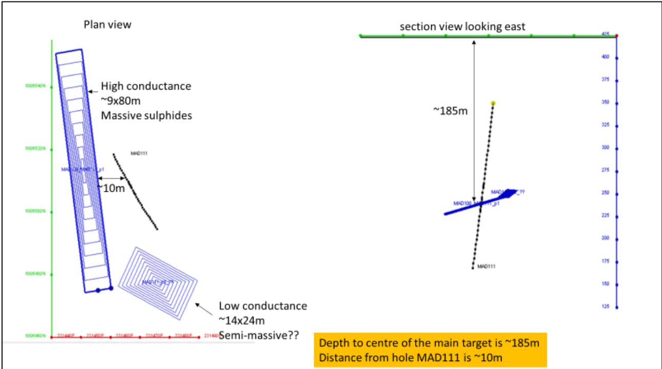
Figure 1 – modelling of the new MAD111: X1 conductor which is 10m to the west of MAD111 and remains untested by drilling.
