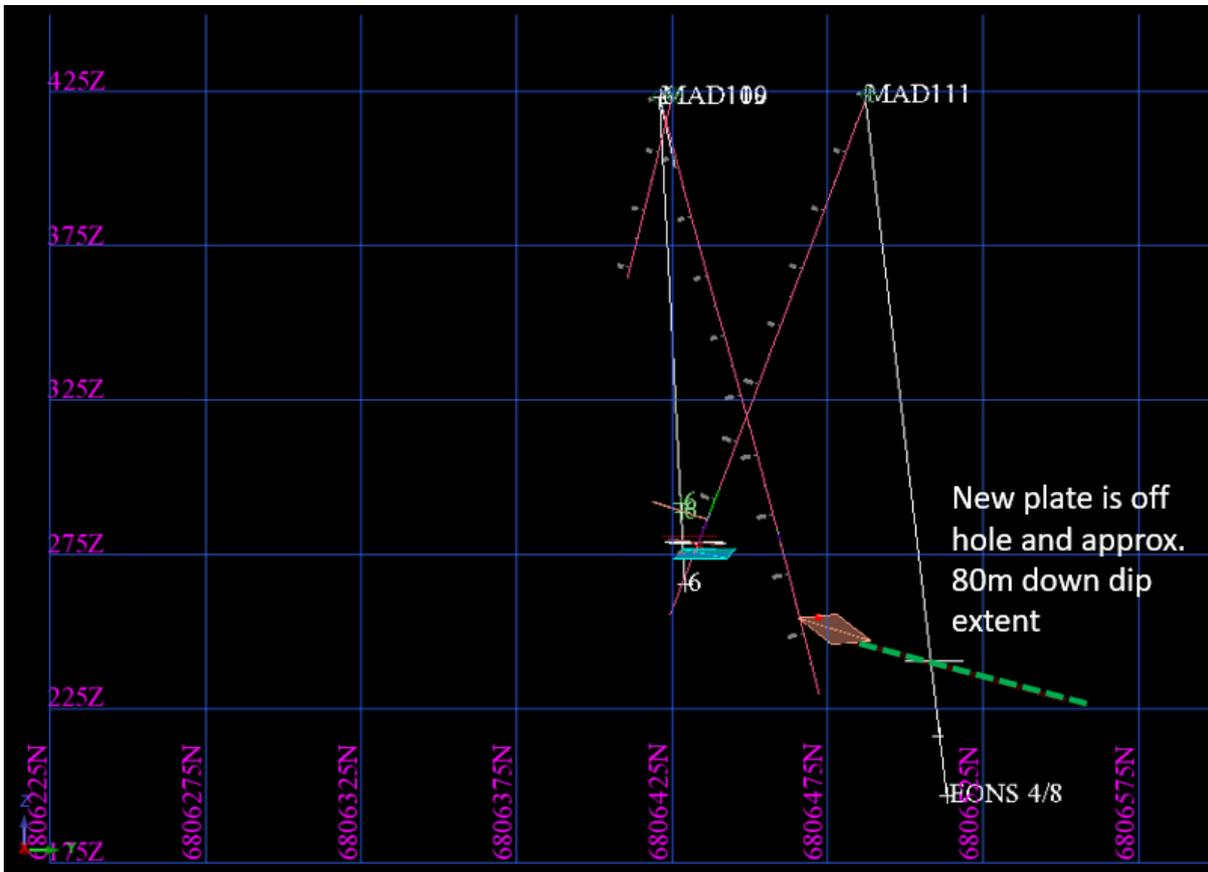
Figure 2 - Section 231460 +/-40m (looking west) showing extent of new 80m plate (green). Recently completed drill holes in white with previously drilled holes in red, against 50m grid squares. MAD111 is 10m to the west of the new conductor and did not intersect it.
