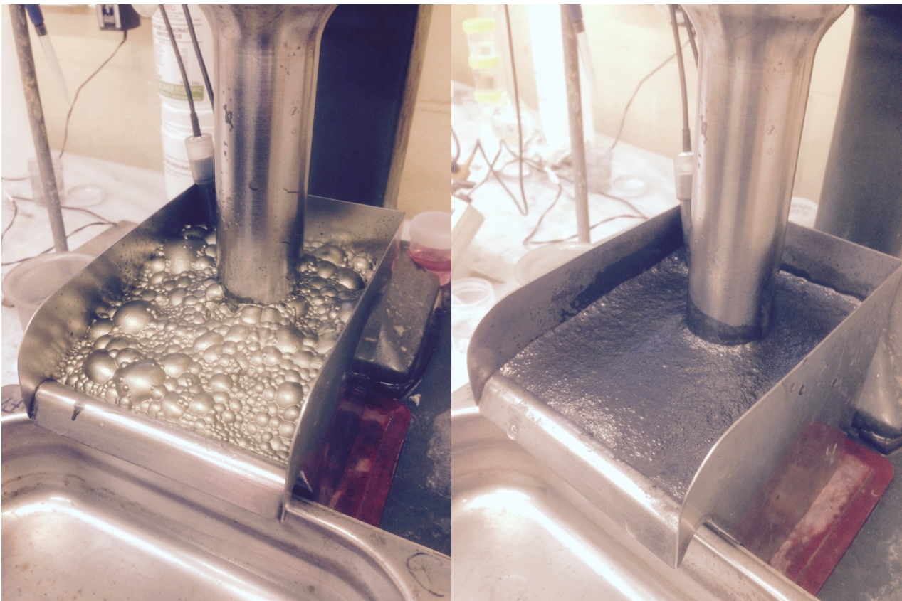
Figure 1 – photographs of a metallurgical flotation test on the Mt Alexander massive sulphide. On left: copper flotation test, with concentrates up to 32%Cu produced. On right: nickel flotation test, with concentrates up to 18%Ni produced.
