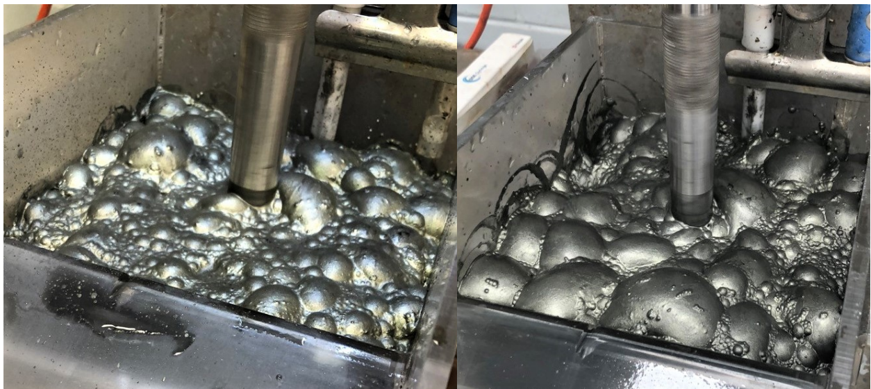
Figure 2 – photos of flotation tests for massive sulphides: on left – copper flotation; on right – nickel flotation.
