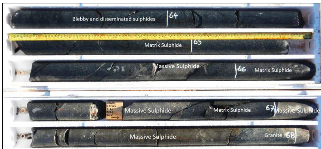
Figure 3 – photograph of drill core from MAD59 between 63.5m to 68.05m including massive sulphides.
