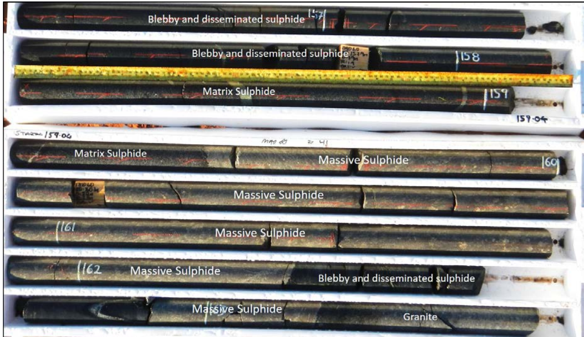
Figure 1 – photograph of drill core from MAD60 between 156.4m to 163.6m showing thick massive nickel-copper sulphide.
