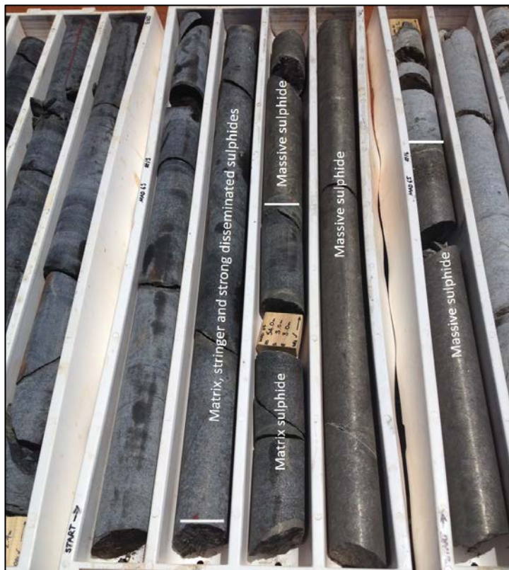
Figure 2 – core tray from MAD65 showing Ni-Cu sulphide mineralisation
