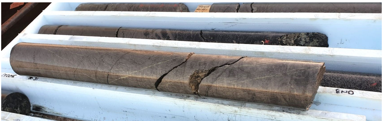
Figure 1 – drill core tray for STD015 showing massive sulphides intersected from 67.3m downhole.
