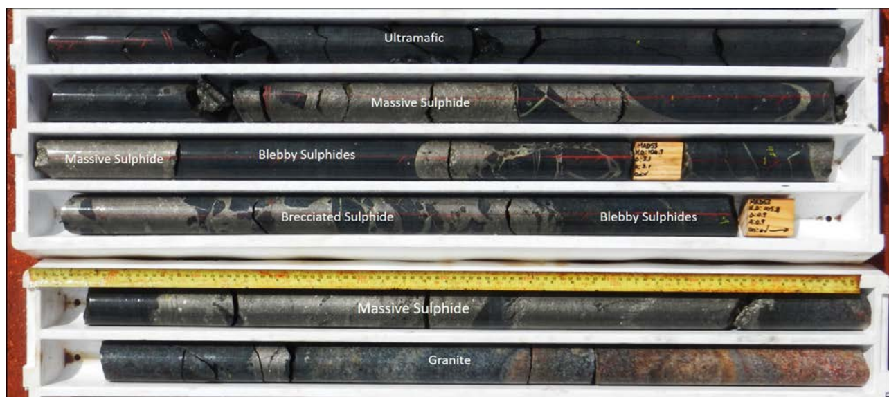
Figure 1 – photograph of drill core from MAD53 between 102.4m to 107.7m including massive, brecciated and blebby nickel-copper sulphides.
