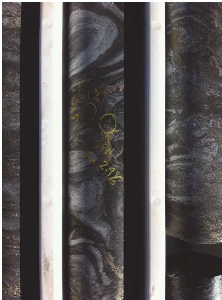
Figure 1 – a photo of drill core from DDRDD0005 at approx. 296m downhole. Chalcopyrite and sphalerite are visible in this sulphide rich interval. XRF analysis returned spot values of 2% Cu and 2.9% Zn.
