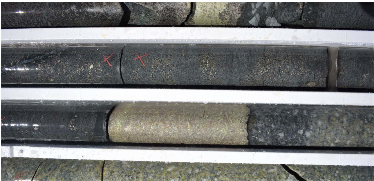
Figure 1 – drill core from MAD173 at approximately 274m downhole showing massive sulphides and heavy disseminated sulphides.
