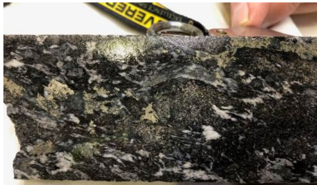
Figure 10 – core from 236m depth within PDD002 completed at the Paterson Project showing disseminated and semi-massive sulphide as void infill within strongly altered breccia.
