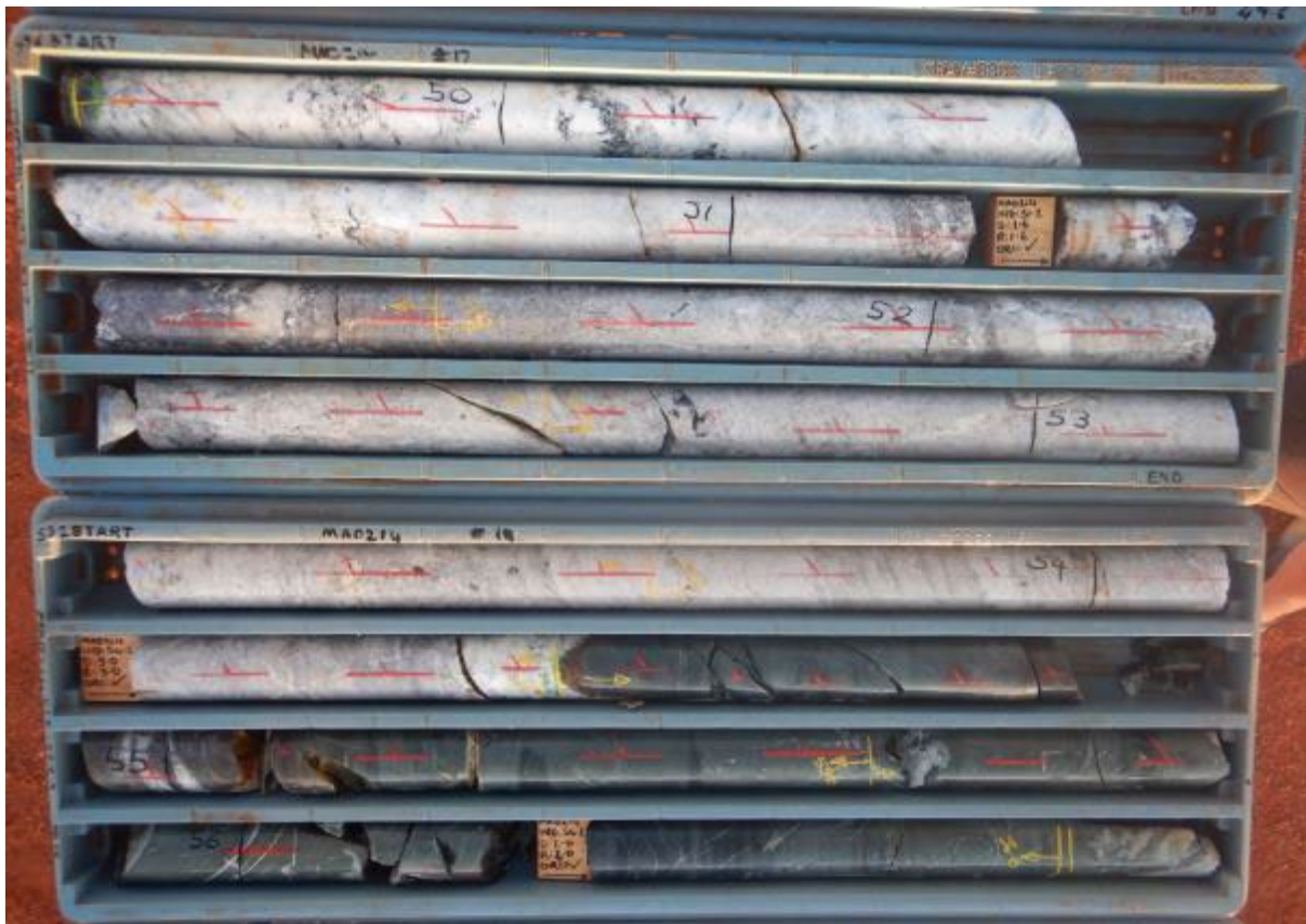
Figure 4 – photo of drill core from MAD214 completed in December 2022 which intersected 5m of pegmatites from 49.5m downhole.
