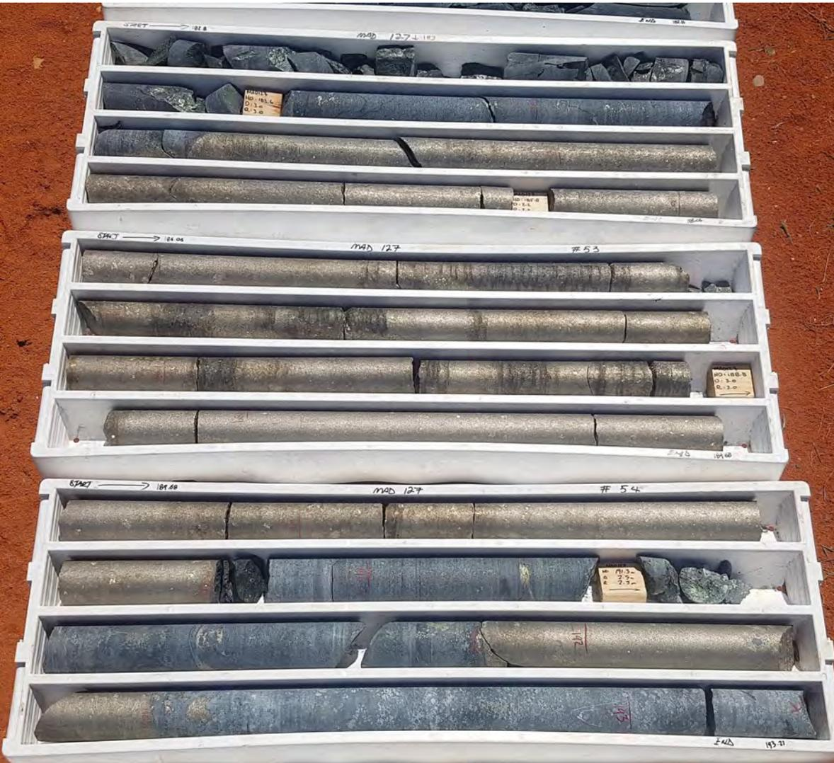
*Right: photo of drill core from MAD136 which intersected 20m of mineralised ultramafic; core shown is from the massive sulphide interval between 149.55m to 151.93m with average XRF readings of 8.1%Ni and 3.21%Cu (assays pending)*
