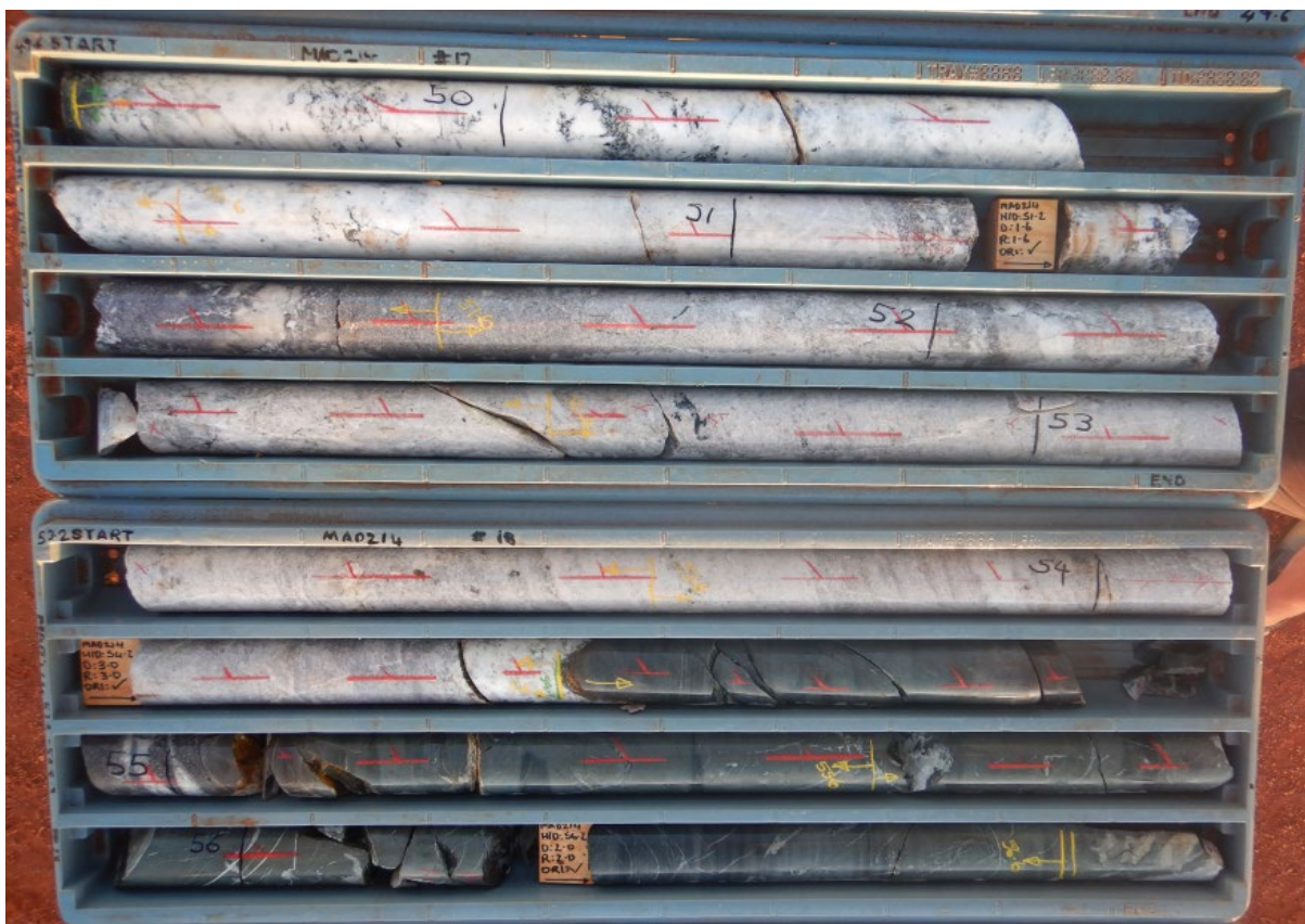
Figure 1 – photo of drill core from MAD214 which intersected 5m of pegmatites from 49.5m downhole.
