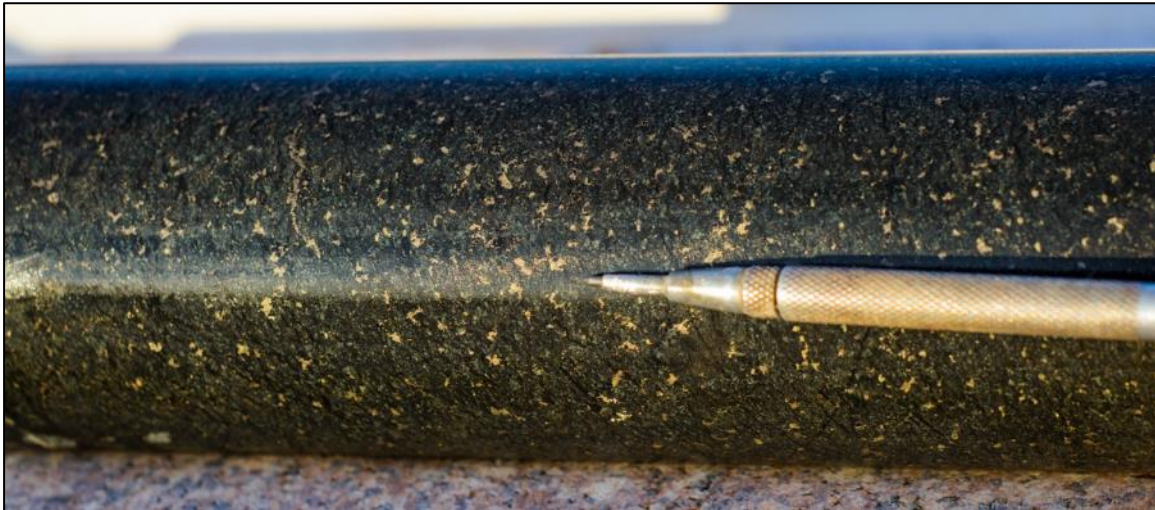
Figure 3 – Drill core with heavily disseminated sulphides from the interval at 46.3m to 48.7m downhole in MAD152 at the Radar Prospect
