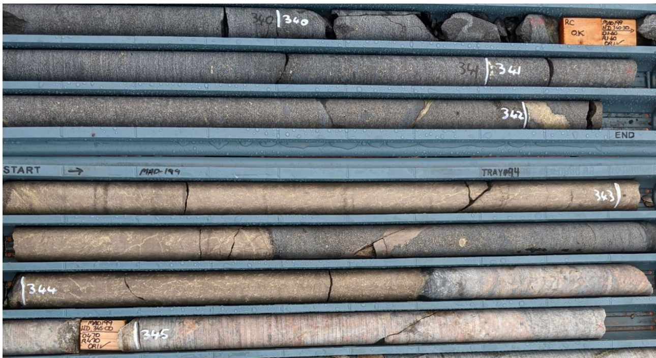
Figure 1 – – drill core tray from MAD199 with the thick interval of nickel-copper sulphides.
