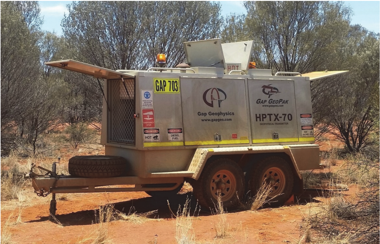
Figure 2 – the HPTX-70 high powered transmitter used for the deep penetrating FLEM SAMSON surveys at Mt Alexander. Field work for 2016 has been completed and the EM crew is scheduled to recommence surveys on 9 January 2017.
