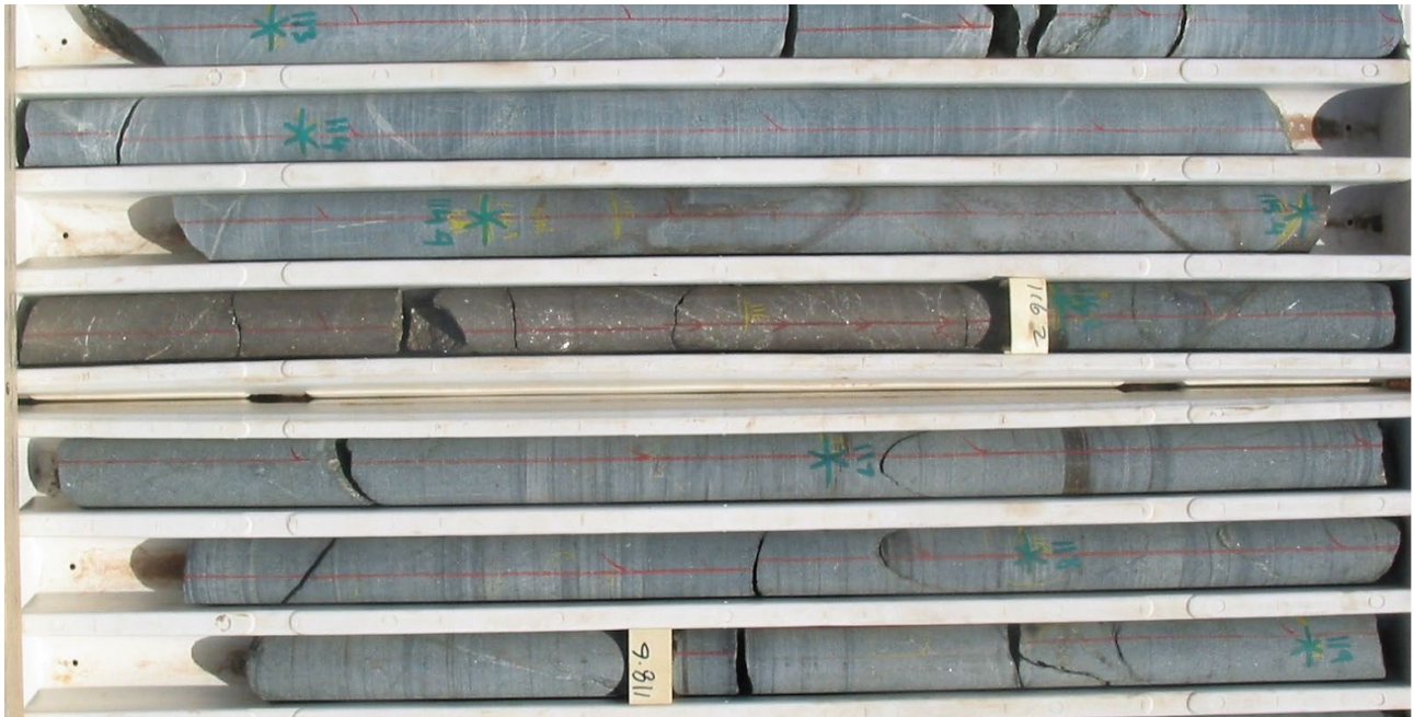
Figure 4 – Diamond drill core from drill hole MAD1. Note the massive nickel sulphides from 115.4m to 116.2m downhole (0.80cm @ 2.57% Ni, 0.13% Cu and 1 g/t PGEs) hosted within meso-cumulate ultramafic rocks.
