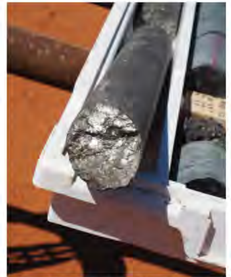
The maiden drill hole at Radar intersected 7.5m of nickel-copper mineralisation, including 2.6m of massive sulphides
