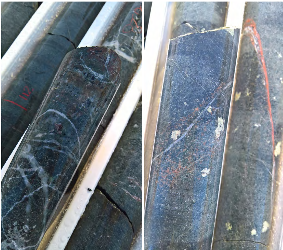
Figure 5 - drill core from ATHDD005 at 113m showing silica – hematite – sulphide altered quartz dolerite, with variable quartz-carbonate veining
