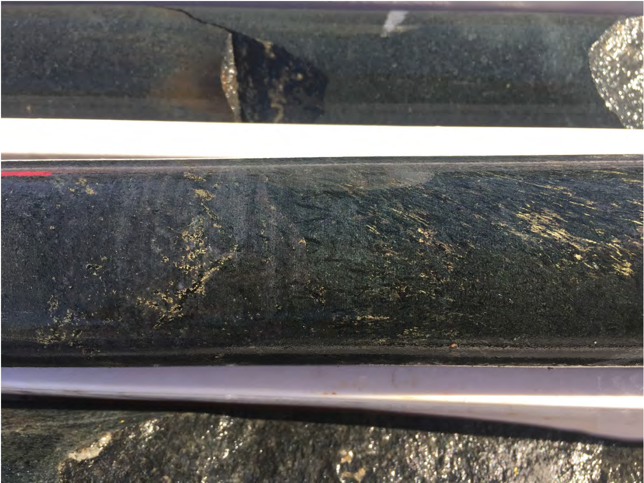
Figure 6 – drill core from ASCDD003 at 117m downhole showing dolerite with pyrite mineralisation
