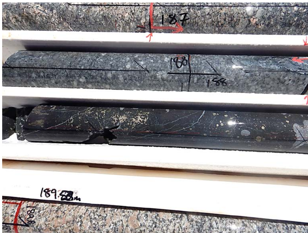
Figure 4 – drill core from MAD118 showing the blebby nickel-copper sulphides in ultramafic
