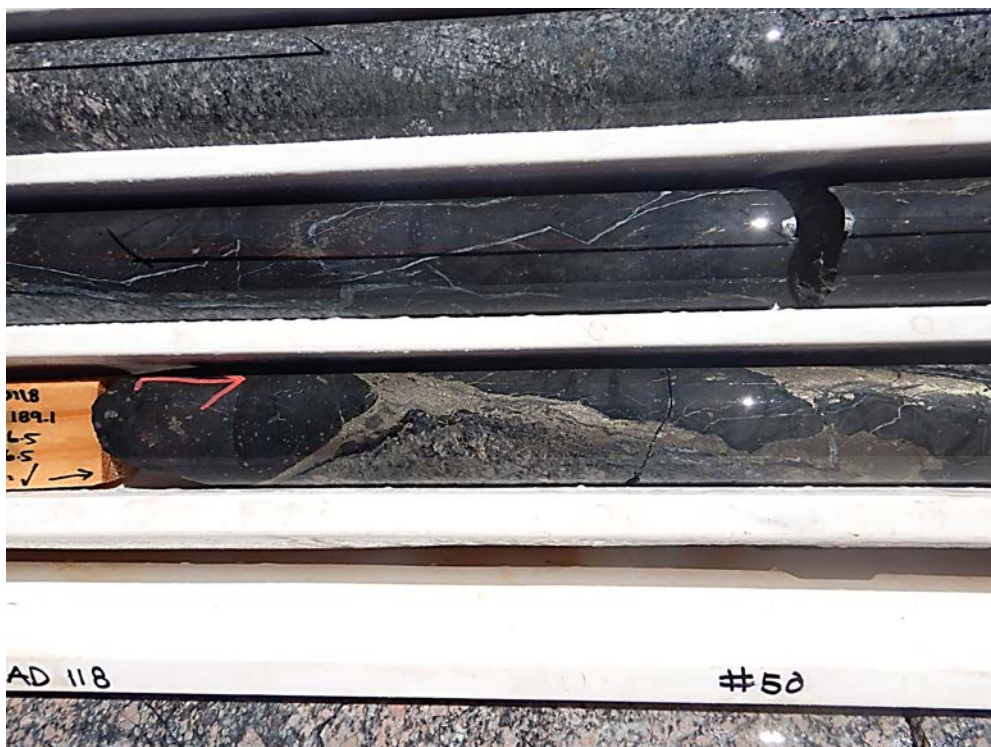
Figure 3 – drill core from MAD118 showing the ribbon of semi-massive nickel-copper sulphides with an unusual high angle (almost vertical) contact
