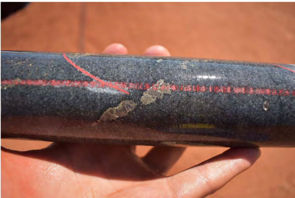
Figure 1 – drill core from MAD172 (approx. 255m downhole) showing heavily disseminated sulphides and large blebby sulphides
