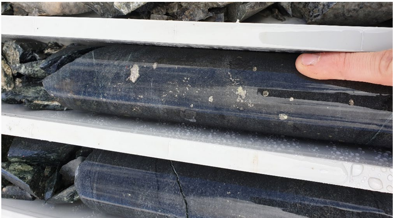
Figure 2 - Photo of drill core from MAD185 showing disseminated and blebby sulphides at about 310m downhole.
