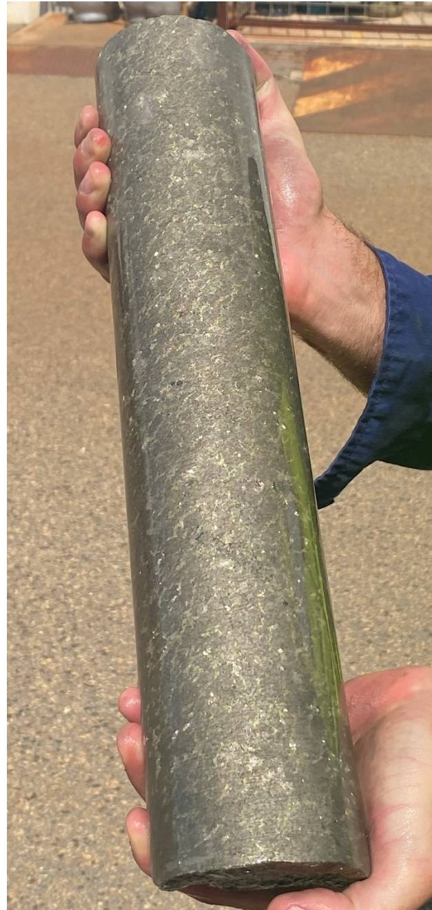
Figure 5 (on right): Photograph of drill core for MAD177 at approx. 185m. Coarse grained pentlandite and chalcopyrite is observed.
