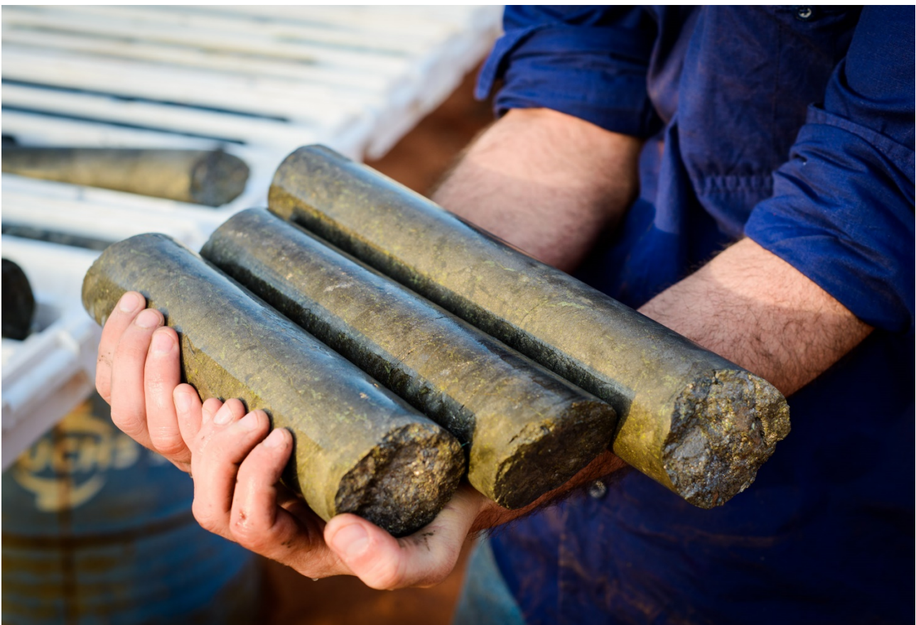
Figure 1 – drill core from MAD152 with massive sulphides that returned assays of 2.55m @ 4.29% Ni, 1.46% Cu and 3g/t PGEs from 49.05m
