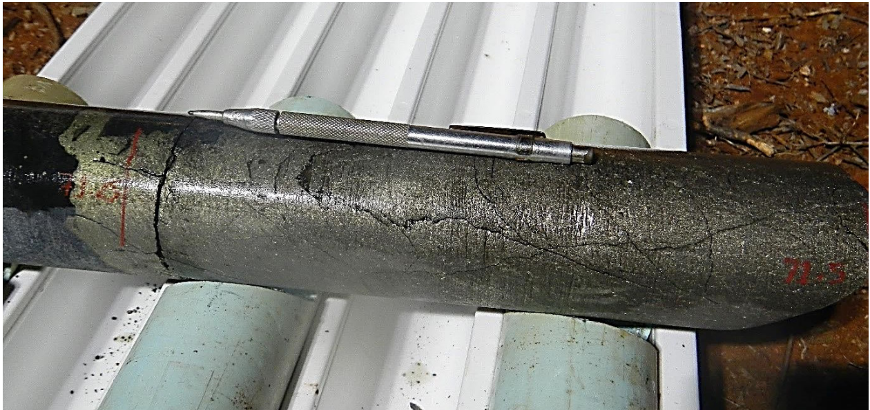
Figure 3 – drill core from MAD27 showing the upper contact of the massive nickel-copper sulphides with the host ultramafic at 71.25m. The massive sulphide averages 4.2%Ni and 2.2%Cu from XRF readings over the 2m interval from 71.25-73.25m.
