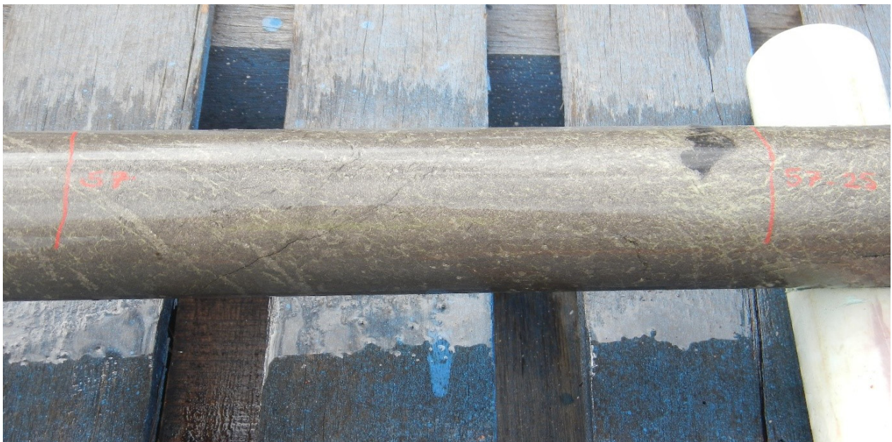
Figure 1 – drill core from MAD26 with massive nickel-copper sulphides at 57-57.25m which recorded spot XRF readings of 8.7%Ni and 2.5%Cu (part of the 2.7m massive sulphide section from 55.2m)
