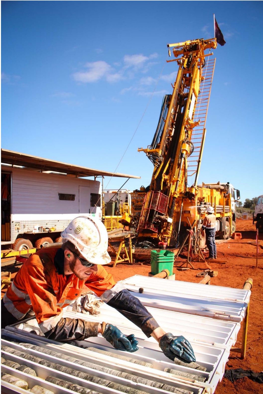
Diamond core drilling at the Desert Dragon nickel prospect in June 2014
