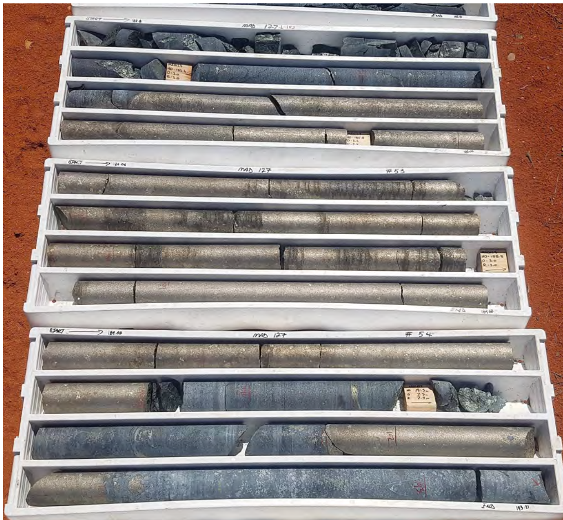
Figure 1 – photo of drill core from MAD127 at the Investigators Prospect that intersected 8.49m @ 5.8% Ni, 2.6% Cu, 0.18% Co and 3.61g/t total PGEs from 183.9m. The next drill programme at Mt Alexander will test new large conductive features at the Investigators Prospect.
