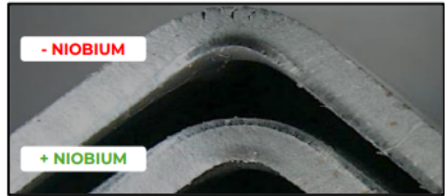
Figure 18: Improved microstructure of steel with Nb additions Figure 19: Improved flat sheet formability with Nb
